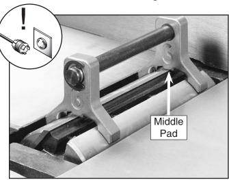
Figure 42. Jig positioned over cutterhead knife.
